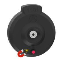
When the device is switched on, the LED flashes once every second for the first 5 minutes, then once every minute. Switch off the unit by sliding the magnet near the power symbol
